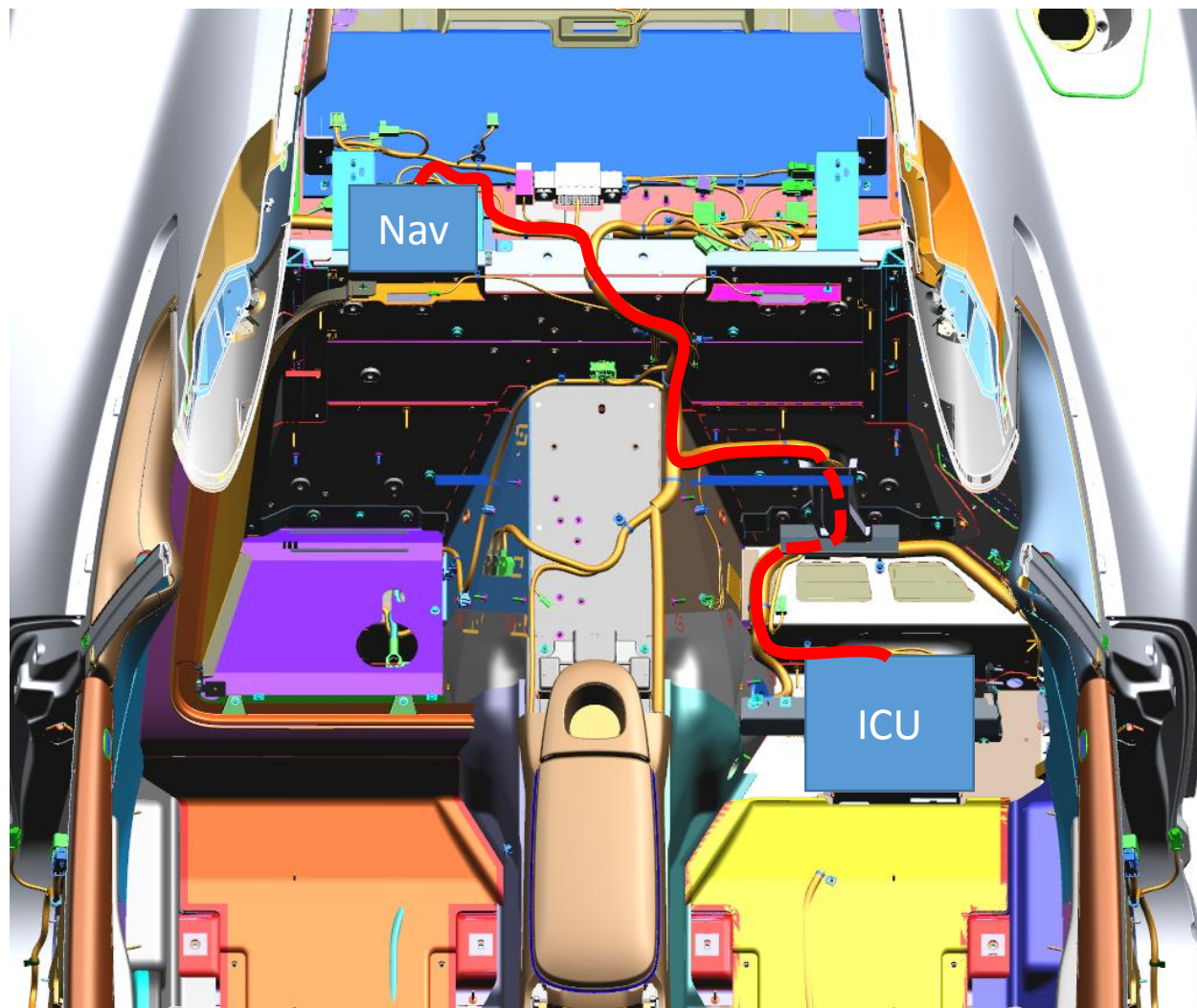
Figure 3 – Advised GPS link lead routing. (NB: Parcel shelf removed for clarity of diagram)
