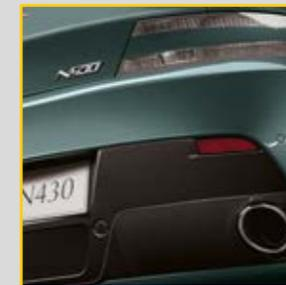
Carbon-Fibre rear diffuser
