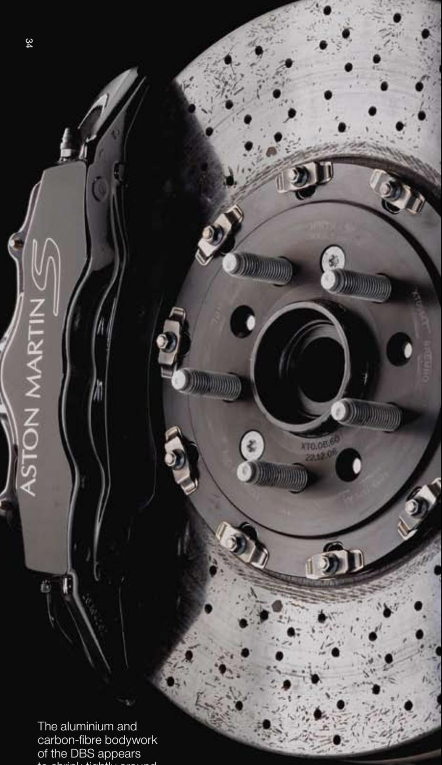
The aluminium and carbon-fibre bodywork of the DBS appears to shrink tightly around the 20" wheels, through which one gets a tantalising glimpse of the car's carbon ceramic brakes, a first for a road-going Aston Martin. These race-bred brakes are lighter, more durable and deliver outstanding stopping power and fade resistance.
